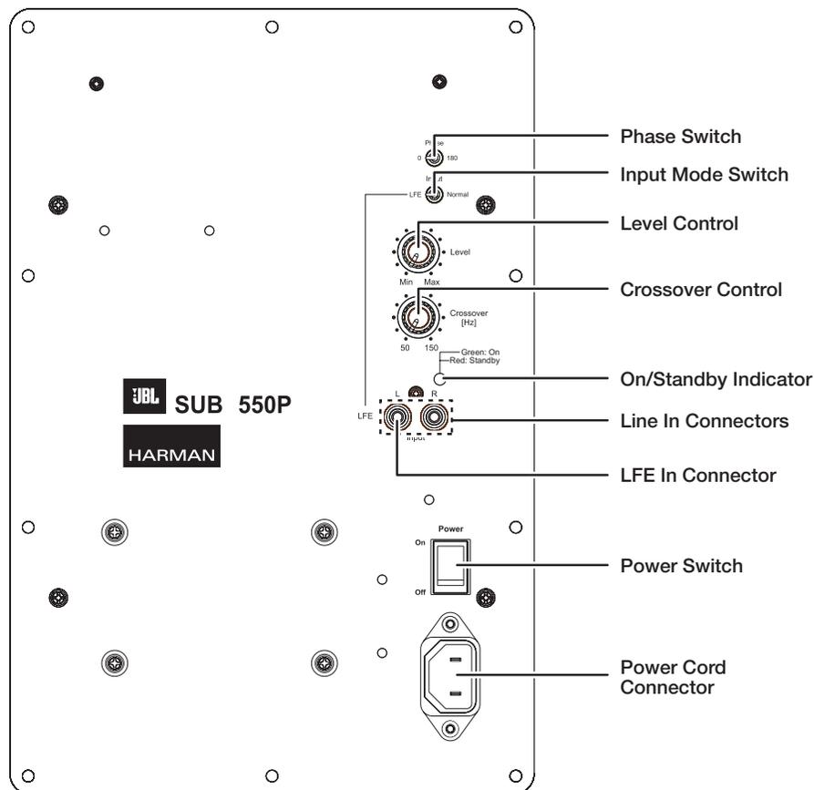
**Phase switch:** This switch determines whether the subwoofer driver's piston-like action moves in and out in phase with the system's other speakers. If the subwoofer were to play out of phase with the other speakers, the sound waves from the other speakers could partially cancel out the sound waves from the subwoofer, reducing bass performance and sonic impact. This phenomenon depends in part on the placement of all the speakers relative to each other in the room.
