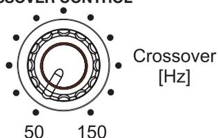
The Crossover control adjusts the subwoofer's built-in crossover between 50Hz and 150Hz. The higher you set the Crossover control, the higher in frequency the subwoofer will operate and the more its bass will "overlap" that of the satellite speakers. This adjustment helps achieve a smooth transition of bass frequencies between the subwoofer and the satellites for a variety of different rooms and subwoofer locations.
