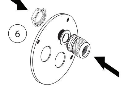
Attach one of the two included Gland Nuts into the open hole on the seal plate as shown above.
