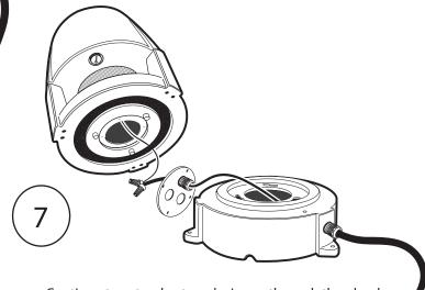
Continue to extend external wire up through the gland nut installed on the seal plate and attach to pre-existing wires from the top section of the speaker with included gel-filled wire nuts.
