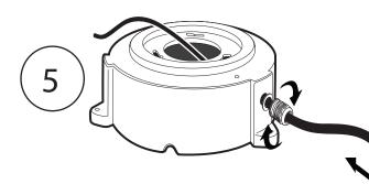
Install the gland nut into the hole as shown above in #6 and feed external wire from outside through the gland nut and up through the center hole in the lower half of the speaker as shown above.
