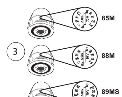
Close-up view of tap setting for the Control 85M, Control 88M, and Control 89MS. \*\*Adjusting tap setting required before powering up system.
