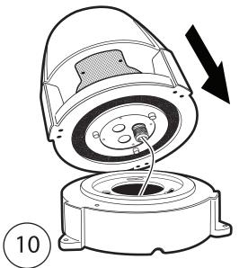
Line up the upper section pins and lower section grooves.
