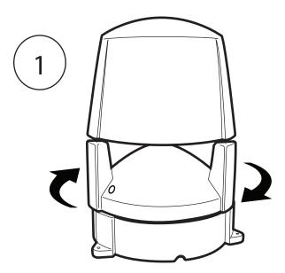
Twist the top part of the enclosure in a clock-wise direction until it disengages from the bottom part.
