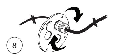
When all wires are set into place as shown in #9, tighten down both gland nuts by rotating the larger side until the gland material clamps down on the wire creating a water tight seal.
