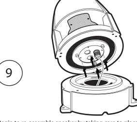
Begin to re-assemble speaker by taking care to place wire nut connectors in top section of speaker and reattach the seal plate with screws as shown above.
