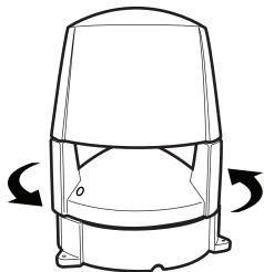
Rotate top section counter-clockwise to lock the top to the bottom section, being careful to line up the security screw hole with brass nut on the bottom half of the speaker.
