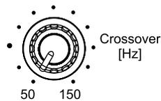
The Crossover control adjusts the subwoofer's built-in low-pass filter crossover between 50Hz and 200Hz. The higher you set the Crossover control, the higher in frequency the subwoofer will operate and the more its bass will "overlap" that of the satellite speakers. This adjustment helps achieve a smooth transition of bass frequencies between the subwoofer and the satellites for a variety of different rooms and subwoofer locations.
