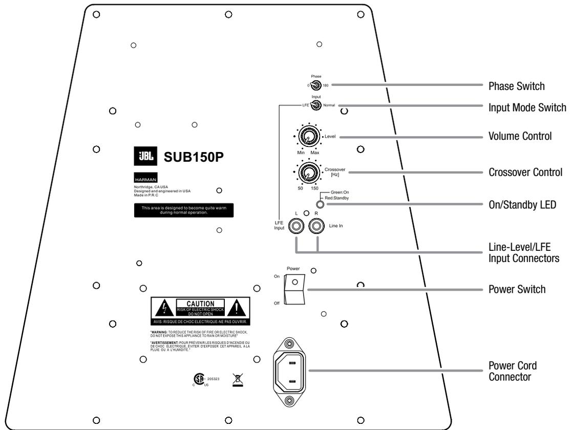
**Phase Switch:** This switch determines whether the subwoofer transducer's piston-like action moves in and out in phase with the main speakers. If the subwoofer were to play out of phase with the main speakers, the sound waves from the main speakers could partially cancel out the sound waves from the subwoofer, reducing bass performance and sonic impact. This phenomenon depends in part on the placement of all the speakers relative to the listening position and to each other in the room.
