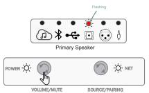
The 4305P system will enter low power standby mode automatically when no signal activity is detected at the active / selected source for >10 minutes.
